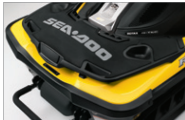
Reboarding platform with storage
