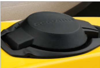
Quick latch fuel filler design
